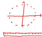
But wait... wouldn't the ruler expand? Not really. Our analysis used the geodesic equation for free test particles. The bits of the ruler are not free but also experience electromagnetic binding forces which swamp the puny gravitational distortion. So yeah, a ruler will do the trick.
